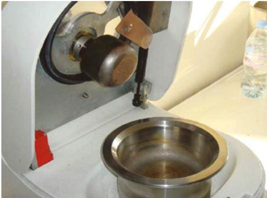
Fig. 1: PULVERISETTE 2 with Mortar bowl made of stainless steel
